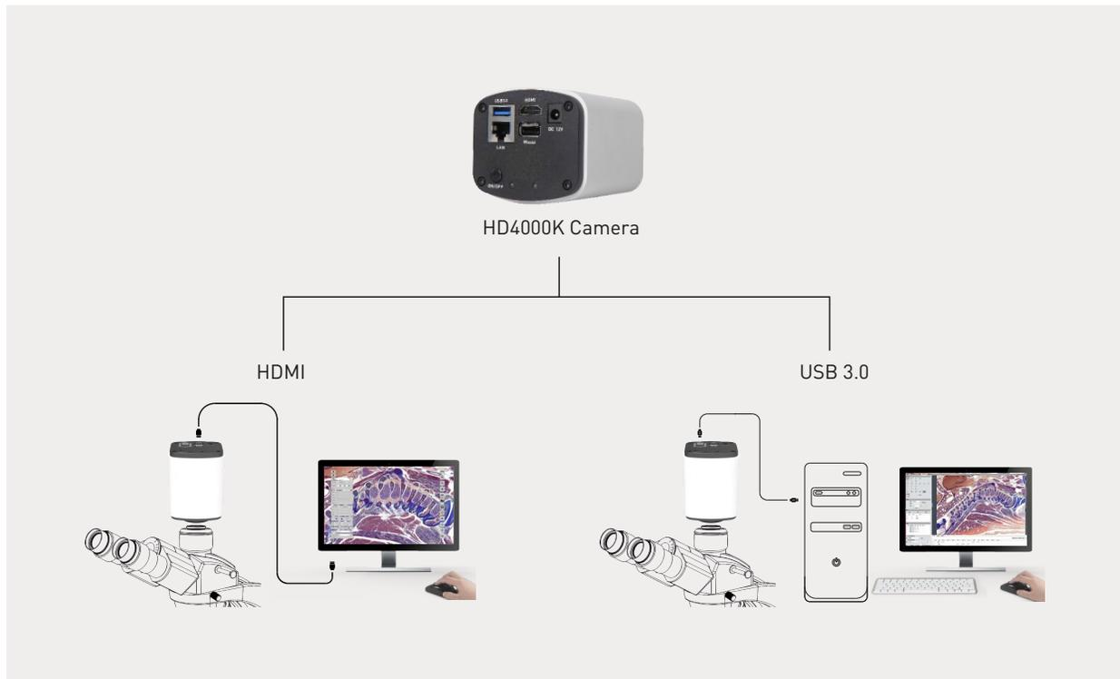
HD4000K and HD4000K-M are microscope cameras that have HDMI and USB 3.0 connectivity and contain professional software analysis.
