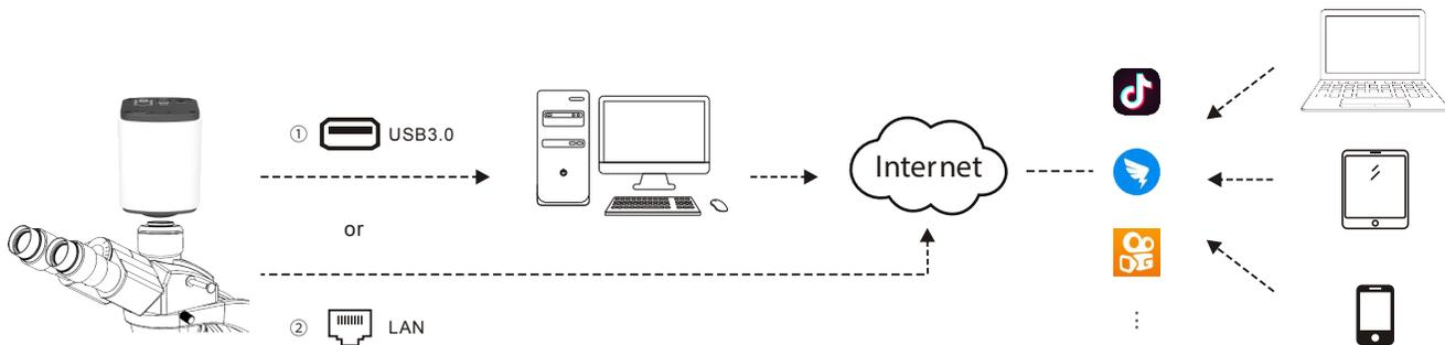
Note: ① USB 3.0: can perform voice interaction under the help of computer audio function.
